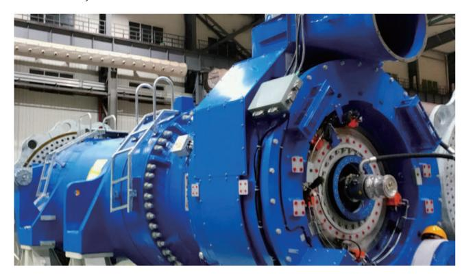
• Wolong developed 3 MW permanent magnet direct drive wind turbines for domestically well-known wind turbine manufacturers
