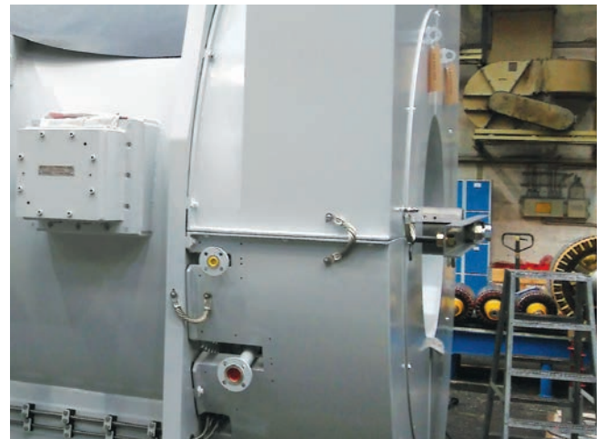
Fan cover with noise reduction measures
