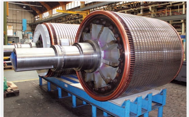
Rotor with copper cage winding
