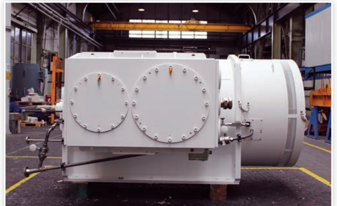
Drive for pipeline oil pump, Ex db (eb) IIB T4 Gb, 1.350 kW, 6 kV, 2-pole; bearings with force-feed lubrication.
