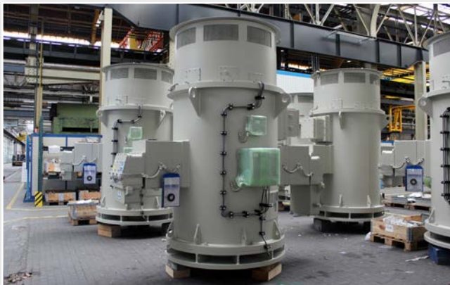
Drive for vertical pipeline oil pump, Ex db (eb) IIC T4 Gb, 600 kW, 3,3 kV, 6-pole; ambient temp. +58°C, bearings with force-feed lubrication.
