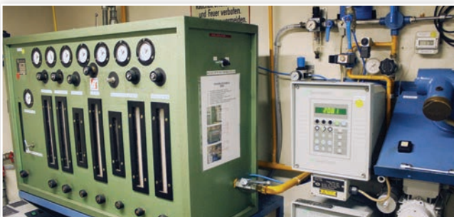
Equipment for mixing and monitoring the gas- air mixture
