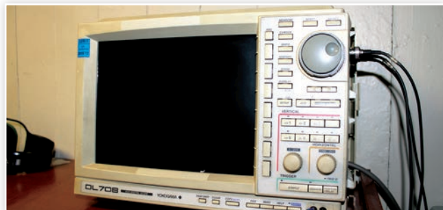
Evaluation of transient explosion pressures
